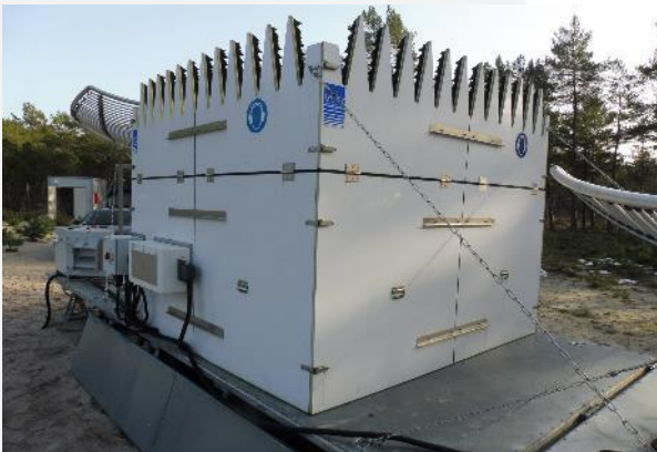
Sodar (sound detection and ranging)
